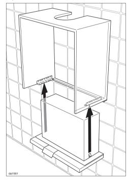
Lift the appliance up into the housing from below, and engage in the brackets.
